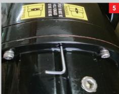
Tighten the M5 socket set screw on gear housing with a 2.5mm Allen wrench to retain the clutch.
