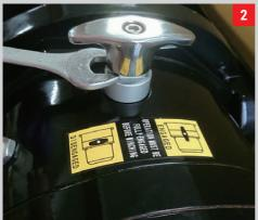
HV-8/HV-10 Pull up on the T-handle and use a 22mm wrench to unscrew the T-handle assembly from the gear housing.
