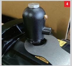
Rotate the air clutch assembly counter clockwise to locate the air port in the desired orientation. Do not unscrew the air clutch assembly more than one full revolution to orient the air port.
