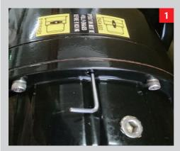
Using a 2.5mm Allen wrench loosen the M5 socket set screw retaining the clutch T-handle threads.
