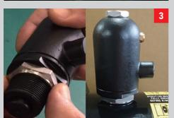
Make sure the 32mm jam nut is threaded to the top of the threads of the air clutch assembly. (HV-8/HV-10 PN: 883226) (HV-12/HV-15 PN: 883227)
