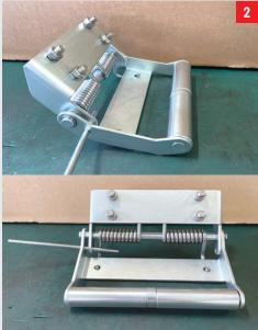
While pushing out the cable tensioner, insert the round bar into the  $\,\phi$  6.4 hole to hold it.
