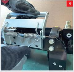
Align to the holes with cable tensioner and winch tie bar. Using a 5mm Allen wrench to secure four M8 screws.
