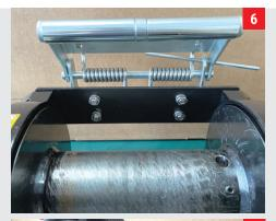
M8 screw and nuts installation complete.
