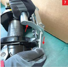
Slightly pull up the cable tensioner and pull out the round bar. Put down the roller with care to avoid finger injury.
