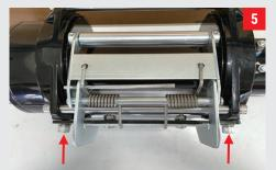
Placing M12 screw into M12 spring washer, and insert it into cable tensioner fixed plate. Secure it with M12 square nut for 2 to 3 circlings.
