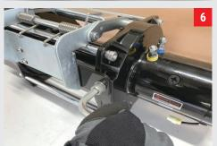
Using a 10mm Allen wrench to secure two M12 screw.
