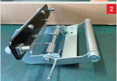
While pushing out the cable tensioner, insert the round bar into the  $\,\phi$  6.4 hole to hold it.
