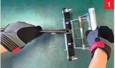
Using an adjustable wrench to push out the cable tensioner.
