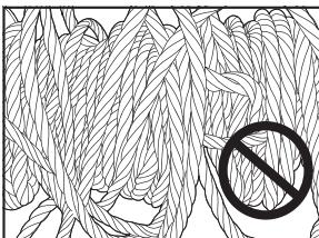
Make sure the rope is wound on the drum evenly. A tightly spiraled pig-tailed rope will damage the rope, shorten its life.
