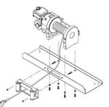
• The wire rope shall be wound in an under-wound orientation only.
