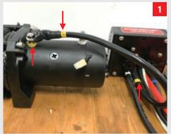
Connect the F1 cable (with a yellow ring on the cable) to the F1 position (with a yellow mark on the motor terminal), then using a 13mm wrench to fasten the nut.
