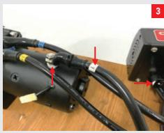
Connect the A cable (with a white ring on the cable) to the A position (with a white mark on the motor terminal), then using a 13mm wrench to fasten the nut.
