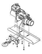
sure the motor, drum and gearbox housing are aligned correctly.
