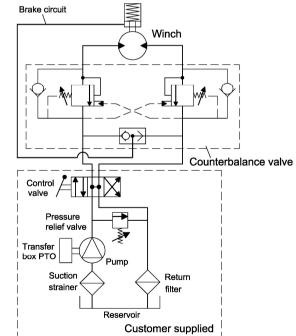
( Powered by PTO / power take off unit driven pump ) The installation of the counterbalance valve supplied is required for 100% braking
