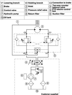
(Powered by PTO / power take off unit driven pump) The installation of the counterbalance valve supplied is required for 100% braking
