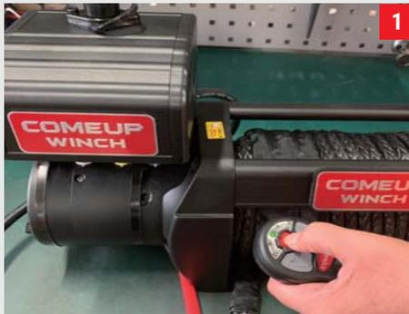
**1 Power on the winch wireless receiver module**
