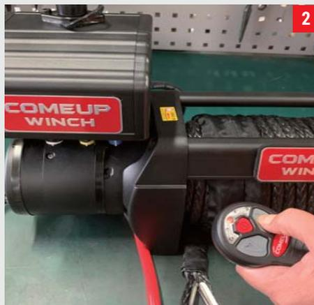
**2 Connect wireless transmitter with winch receiver module**
