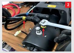
Connect the F1 cable (with a yellow ring on the cable) to the F1 position (with a yellow mark on the motor terminal), then using a 13mm wrench to fasten the nut.
