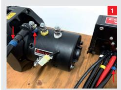
Connect the F2 cable (with a blue ring on the cable) to the F2 position (with a blue mark on the motor terminal), then using a 13mm wrench to fasten the nut.
