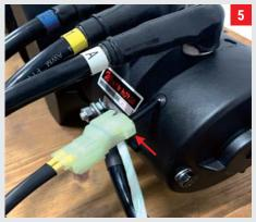
Plug the overheat protector socket of the control box into the overheat protector socket of the motor.
