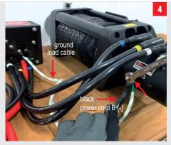
Connect the white ground lead cable (with green tape) and black power cord B (-) to the negative terminal on the motor, then using a 13mm wrench to fasten the nut.
