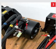
Connect the A cable (with a white ring on the cable) to the A position (with a white mark on the motor terminal), then using a 13mm wrench to fasten the nut.
