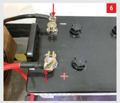
Connect the red power cord (+) of the control box and black power cord (-) to the battery on the vehicle.
